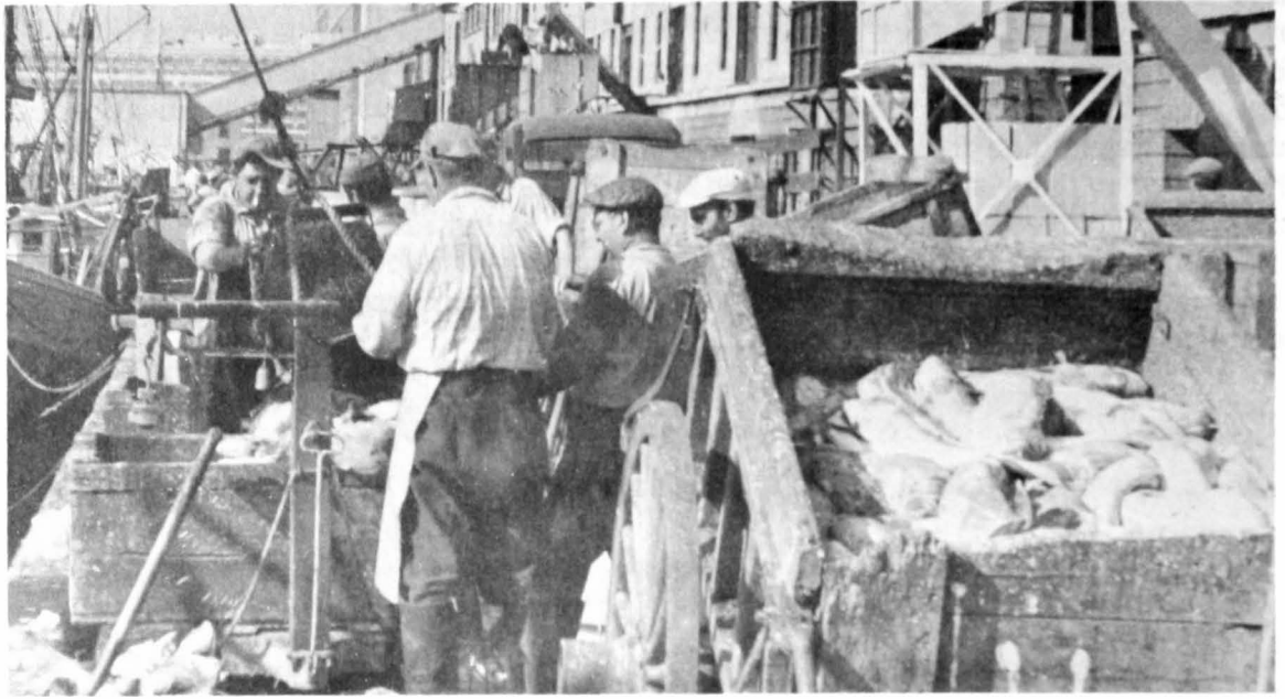
Figure 11.--Dumping fish from a canvas unloading basket into a tared weighing box. A large two-wheeled cart partly filled with fish is shown in the lower right-hand corner.
